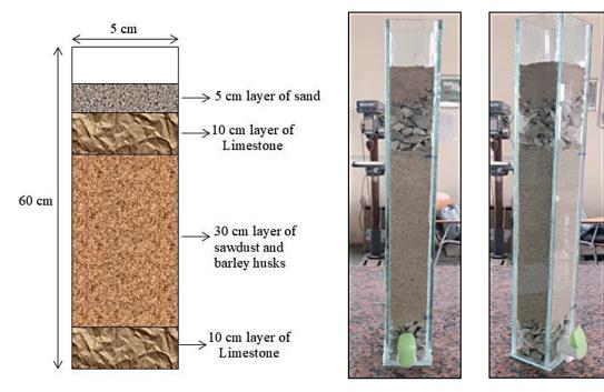
Figure 4. The filter configuration and filter media
