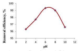
Figure 7. PH effect on the removal efficiency
