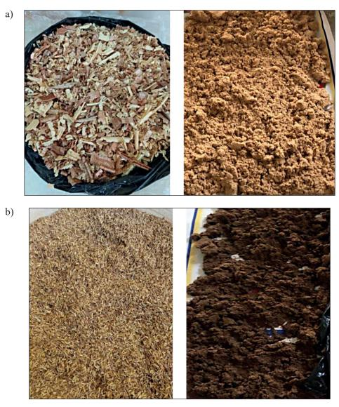
Figure 3. Adsorbents used in the study: (a) saw dust, (b) barley husks
